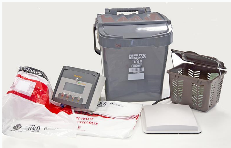
Image 1. Vented kitchen caddy (right hand) and (inside it) compostable bags used for collection of kitchen waste; tagged caddies (centre) and tagged bags (left) adopted to collect residual waste, under a variable charging scheme (PAYT; the delivery of one bag/bucket is detected through receivers and displayed on the square tool).
