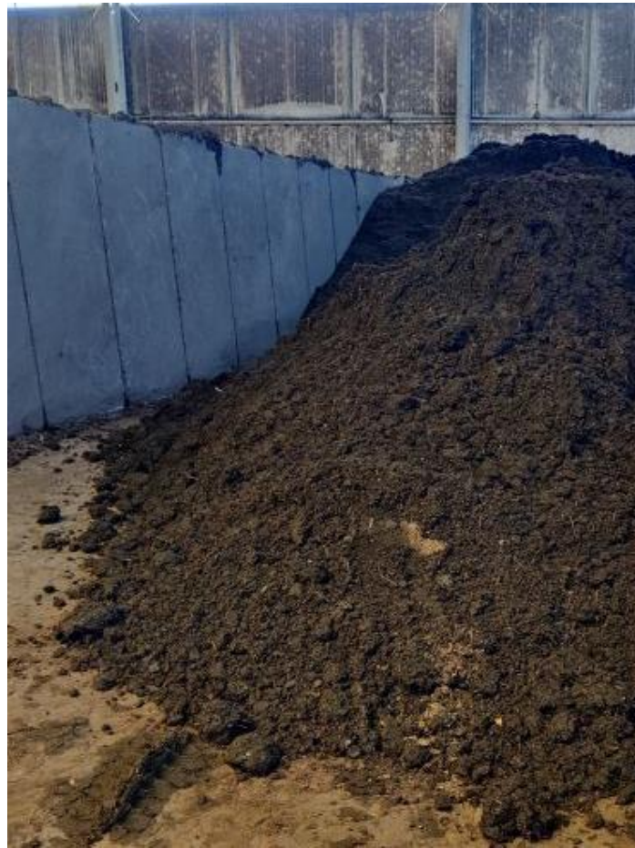
Figure 14. Solid digestate, dewatered after a wet AD process (~35% DM)
