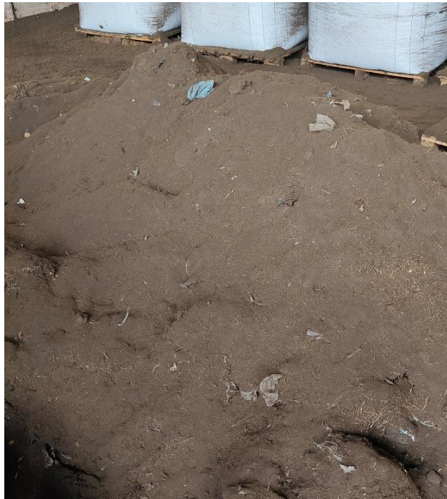
Figure 9. Reject fraction of wind-sifted material
