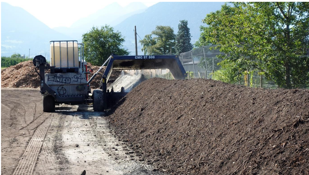
Figure 6. Irrigation on open windrow composting pile
