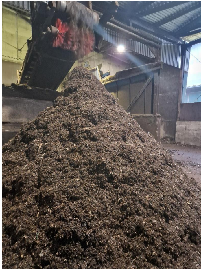
Figure 13. Intermediate 10–30 mm fraction (e.g., sieved by star sieve)
