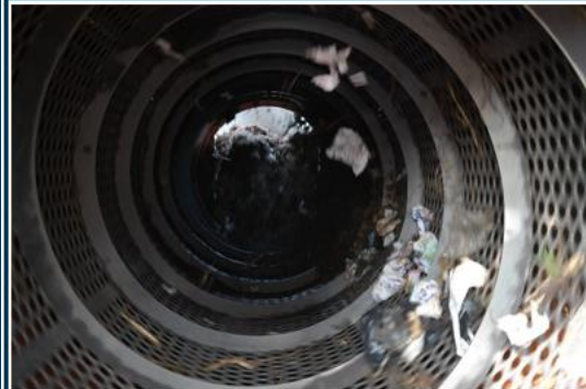
Drum screen for coarse material removal (Siebert, 2014)
