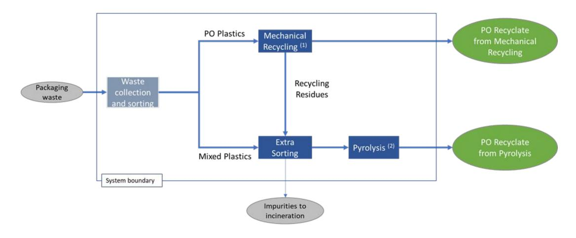
(1) Recycling includes: Washing, further sorting, regranulation. (2) Pyrolysis includes: Pyrolysis, purification of pyrolysis oil, cracking and polymerisation.
