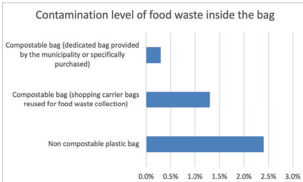
Figure 6: comparison purity/type of bag as assessed by CIC: content of the bag vs. type of bag
