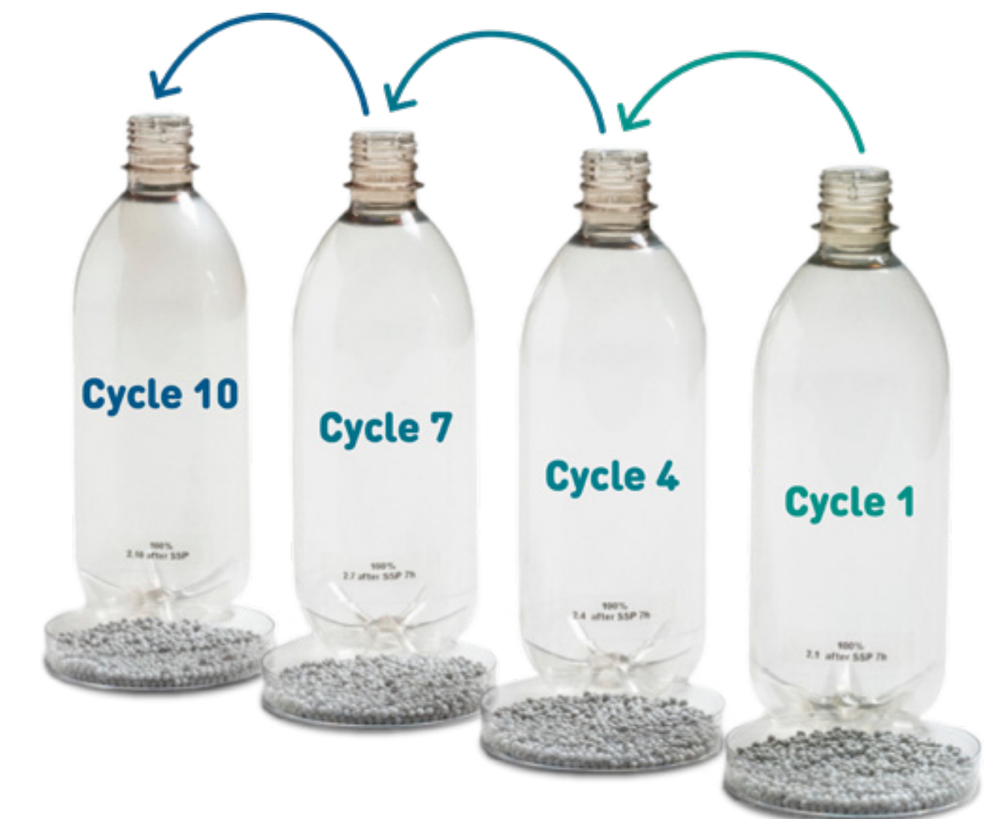
Figure 3.2: Colouration of the bottles blown for successive recycling loops with 75% recycled content [33]
