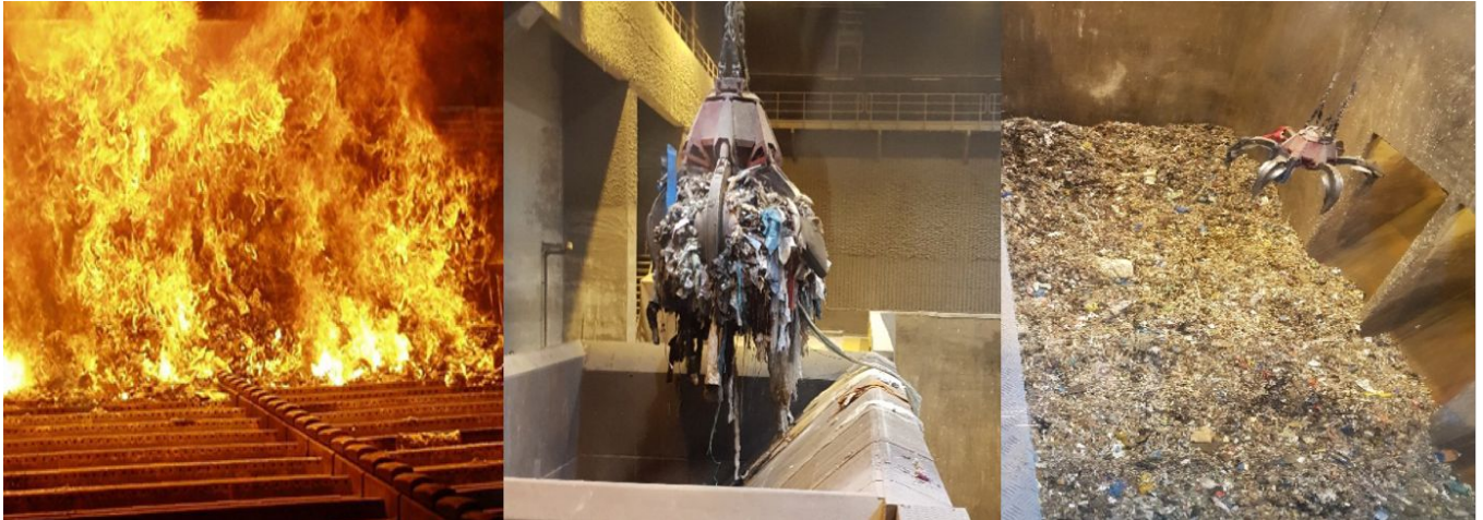
Figure 1 Waste burning at the grid. Waste transported to furnace (photo K. Bouman, 10-12-2019 REC)
