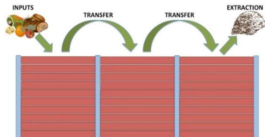
Systems involving two transfers have proved to be the most efficient, as they allocate the different phases of the process to independent spaces, so the required specific parameters for each phase can be met and monitored individually.
