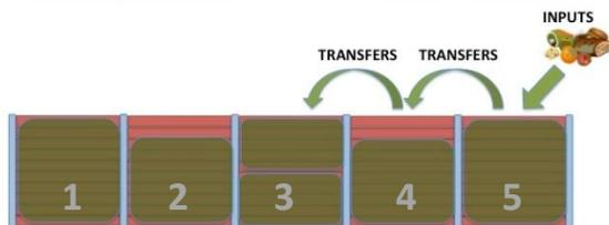
New closedown of module 1 once filled, transfer of material in module 5 to module 4, and module 5 becomes the input module again.
