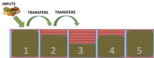
Closedown of module 5 once filled, transfer of material in module 1 to module 2, and module 1 becomes the input module again.
