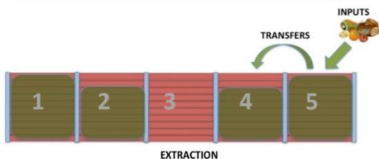
New closedown of module 1 once filled, material transfer from module 4 to 3 and from 5 to 4. New inputs in module 5.
