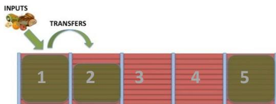
New closedown of module 5 once filled, material transfer from module 2 to 3 and from 1 to 2. Module 1 becomes input module again.
