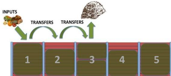
Compost extraction from module 3. Closedown of module 5 once filled, material transfer from module 2 to 3 and from 1 to 2. Module 1 becomes input module again.
